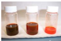
Solutions of nanocrystals blended into a conducting polymer
